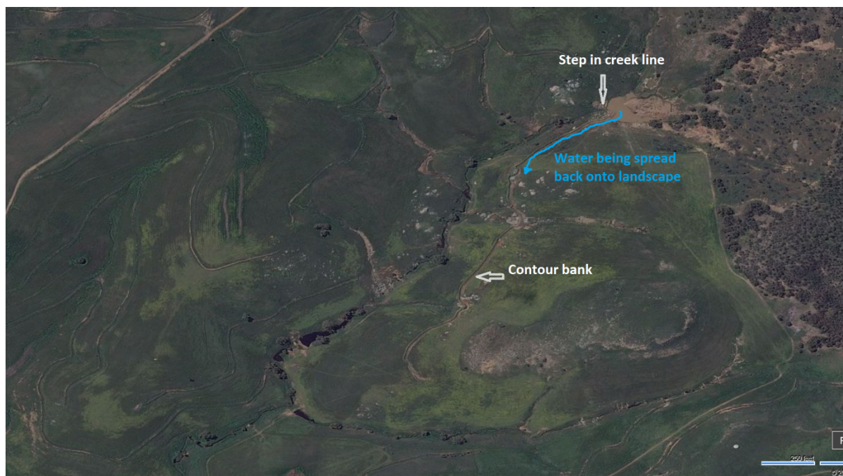
Figure 3 a & b; Constructed earth bank steps (pink) in creeks (blue) where some steps spill water out of the creeks into contour banks (orange) to spread water back across the landscape.
